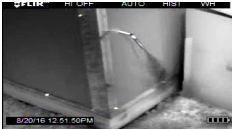
Photo 14. Vent pipe on well Tourmaline DOE 04-11-080-16 W6M venting natural gas to the external environment. This was a continuous flow, measured to be approximately 0.5 m 3 /hr. This is a still photo captured from a video taken with a FLIR camera.
