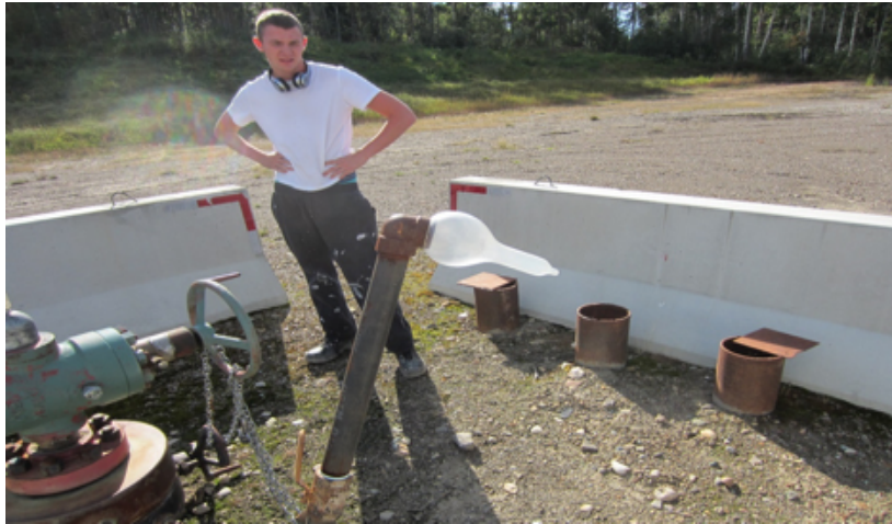
Photo 4. Picture of a balloon applied to the opening of the leaking surface-casing vent shown in Photo 3. The leaking gas has inflated the balloon.
