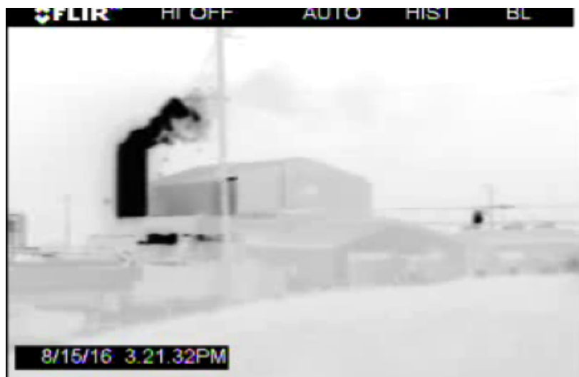
Photo 15. Cloud of heat and methane gas being emitted from Spectra Energy Compressor Station 16 on August 15, 2016. The main plume is probably heat but the residual plume wafting away from the stack is likely unburned gas. The distinct odour of natural gas was very strong at ground level. This is a still photo captured from a video taken with a FLIR camera.
