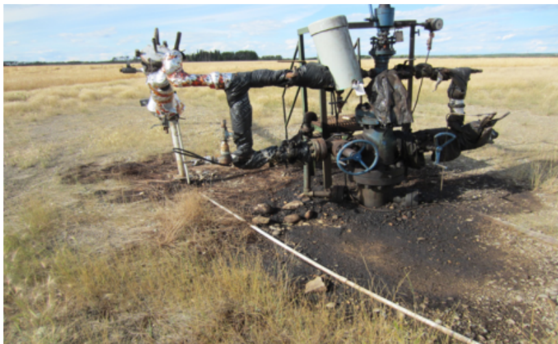
Photo 9. This is well CNRL Owl 08-16-86-18. Note that the entire wellhead and ground around the wellhead are soaked with oil. Photo taken August 19, 2016.
