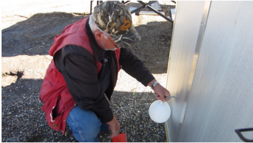
Photo 7. Applying a round balloon to a natural gas vent on the exterior of an instrument shed at an operating gas well site.
