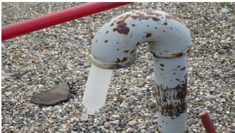
Photo 5. Full inflation of a balloon applied to a surface-casing vent was considered to be achieved when the balloon “snapped to attention” but did not noticeably stretch beyond the dimensions of its resting state.
