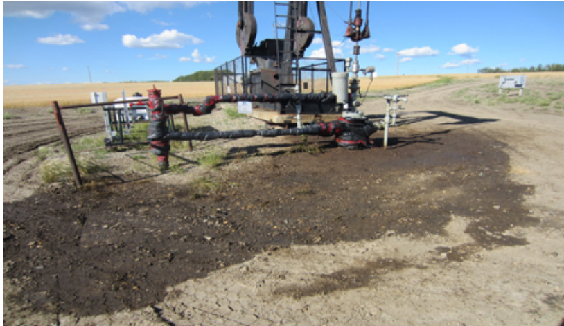
Photo 10. CNRL Eagle A08-07-85-18 appears to have suffered a recent blowout. The entire wellhead and ground around the well are soaked in oil. Photo taken August 18, 2016.
