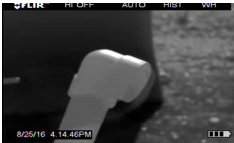
Photo 3. Still image captured from a video of a leaking surface-casing vent. The wisp of grey visible at the opening of the vent is escaping methane gas (as determined using a GEM 2000+ landfill gas monitor).
