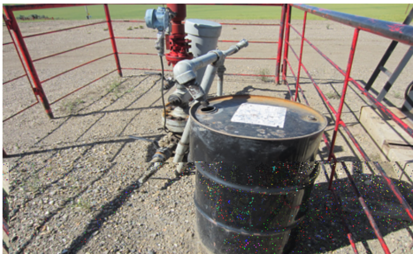
Photo 12. West Eagle 06-11-85-19 w6m. The surface-casing vent on this well was dripping liquid, the flow of which was directed to a 40-gallon metal drum. Photo taken August 19, 2016.
